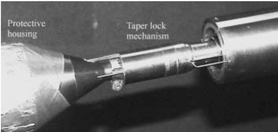
Figure 2: Grinding mechanism in wind-tunnel.
